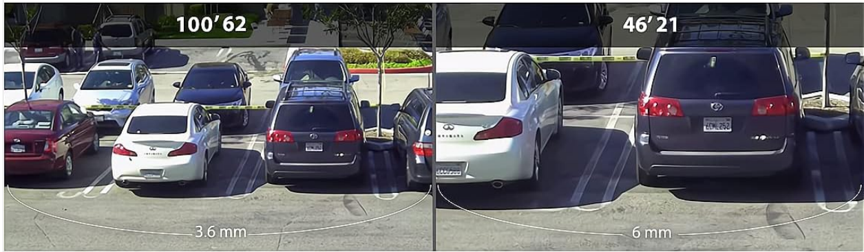
Image 6.6: Comparison of a 3.6mm lens wide-angle view versus a 6mm lens, demonstrating broader coverage.
