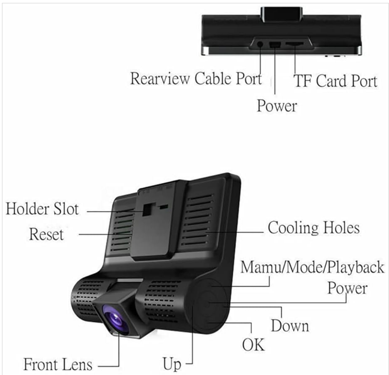
Figure 4.2: Top and bottom views of the dash cam, highlighting various ports and controls.
