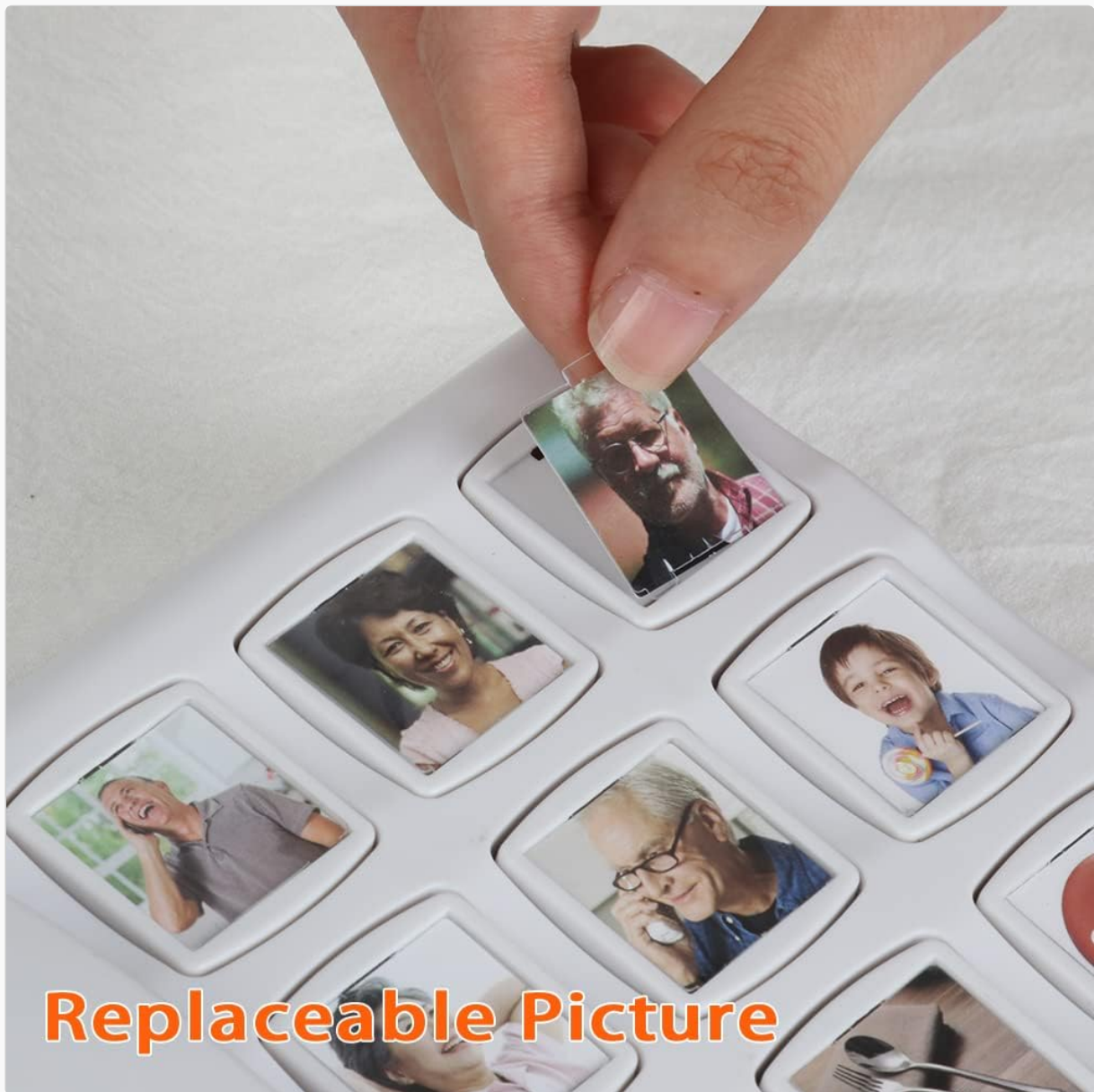
Image 4.2: Demonstrating how to replace the picture inserts on the speed dial buttons.
