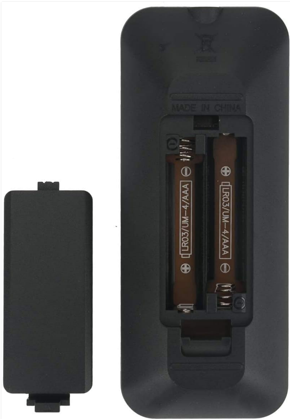
Image: Battery compartment with AAA batteries.
