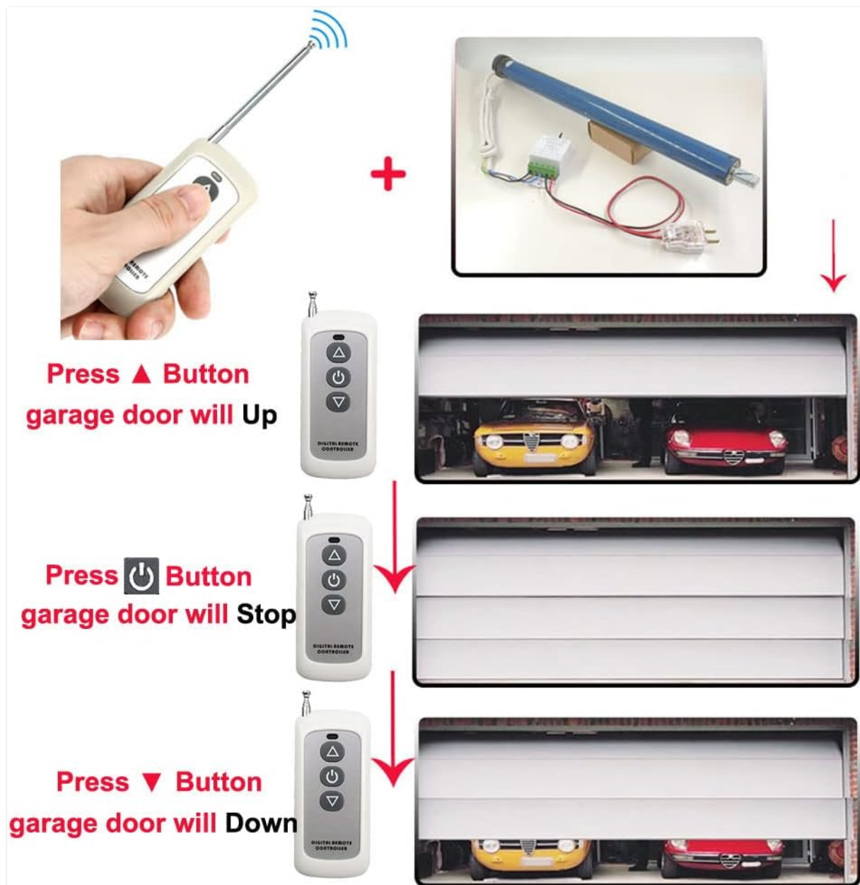
Image 6.1: Controlling a garage door using a 3-button remote in Latched Mode (Up, Stop, Down).
