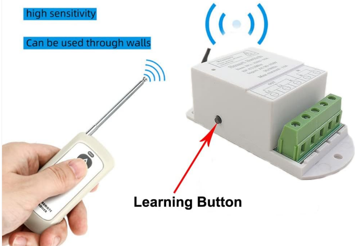
Image 3.1: The wireless receiver module and remote control, showing the learning button on the receiver.
