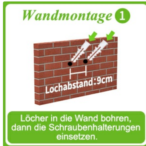
Figure 4: Illustration showing the drilling of two holes 9 cm apart on a brick wall for screw anchors.
