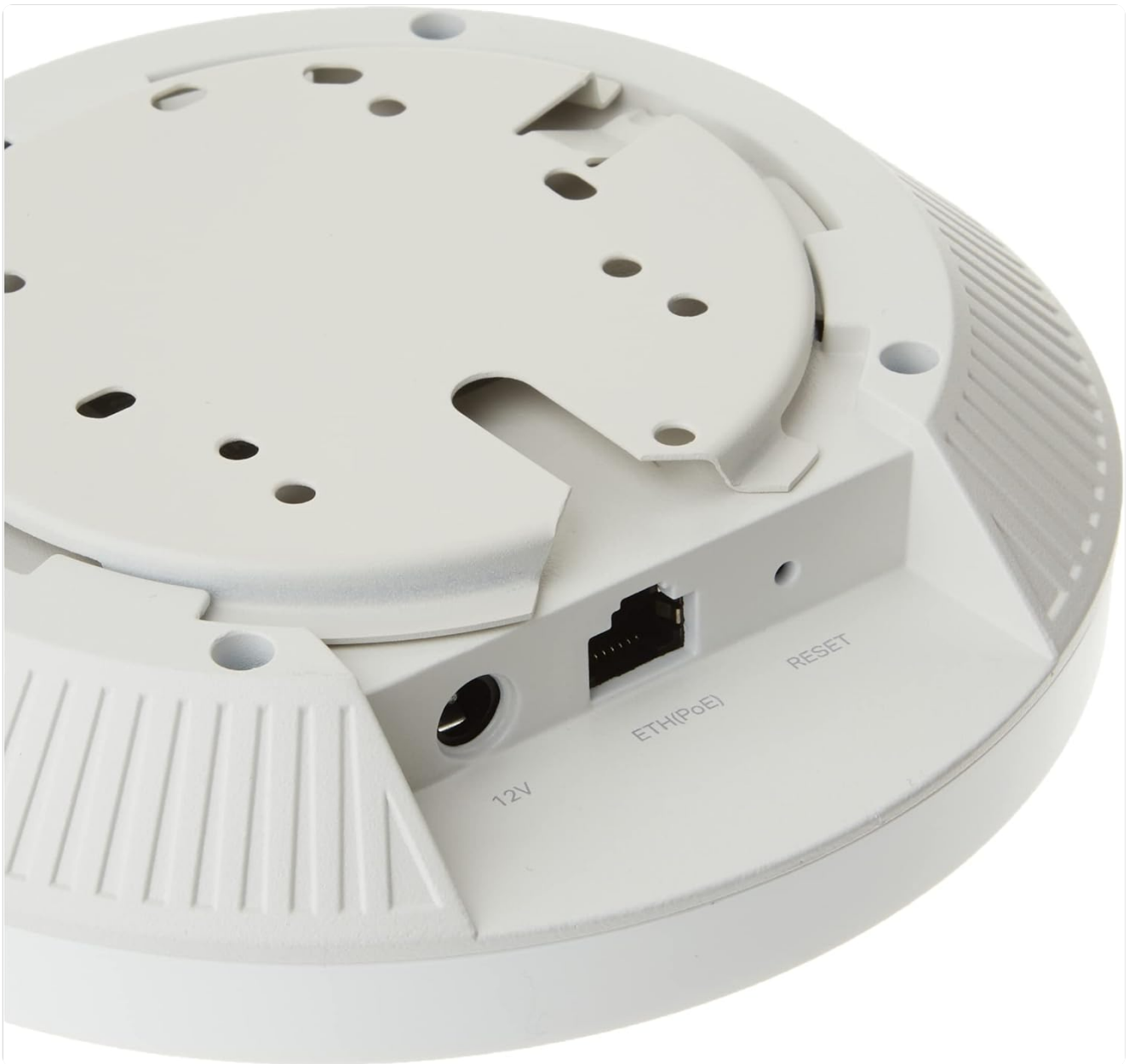
Figure 5: Rear view of the EAP610 V2 showing the 12V DC, ETH(PoE), and Reset ports.
