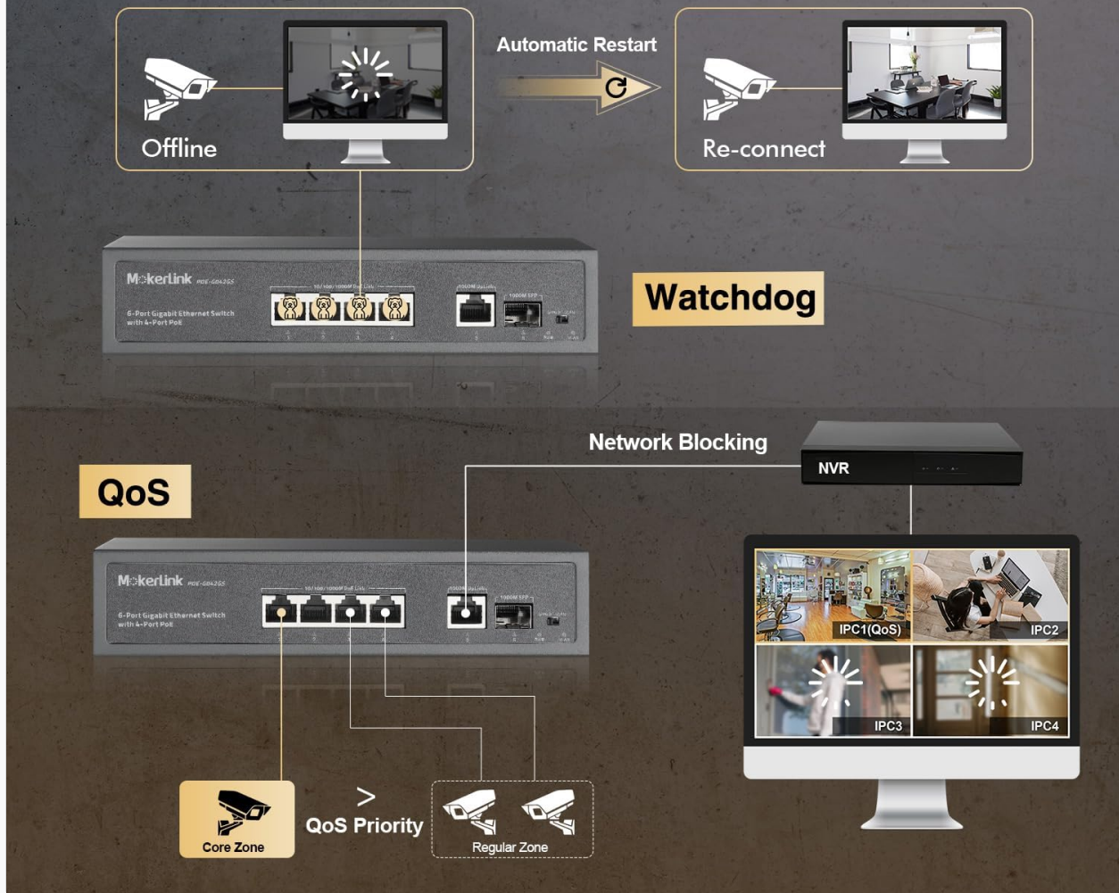
Figure 7: PoE Watchdog and Hardware QoS functions.
