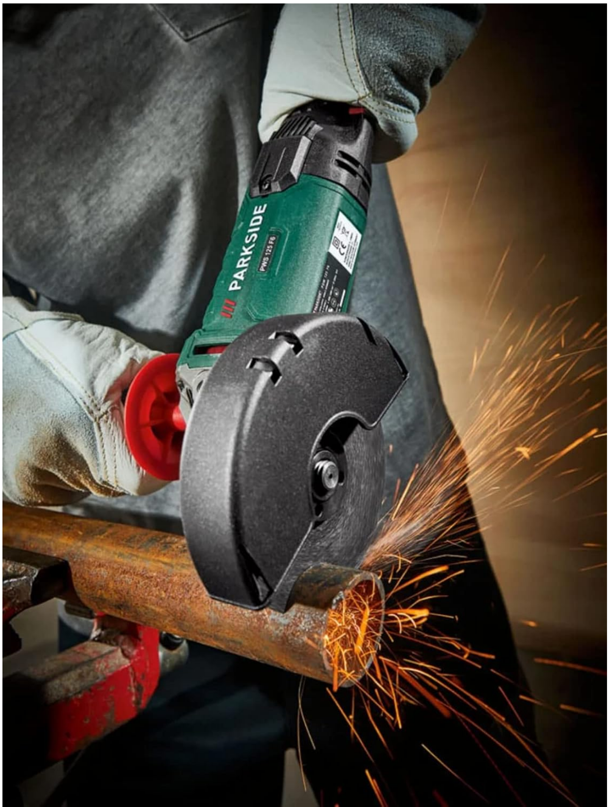
Figure 4: The angle grinder actively cutting a metal pipe, demonstrating proper usage with sparks flying away from the user.
