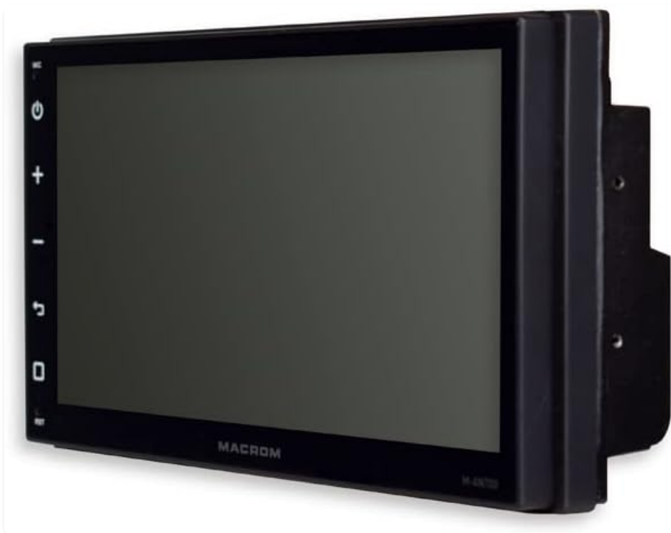
Figure 2.3: Side view of the MACROM M-AN700 car stereo, highlighting its reduced installation depth.
