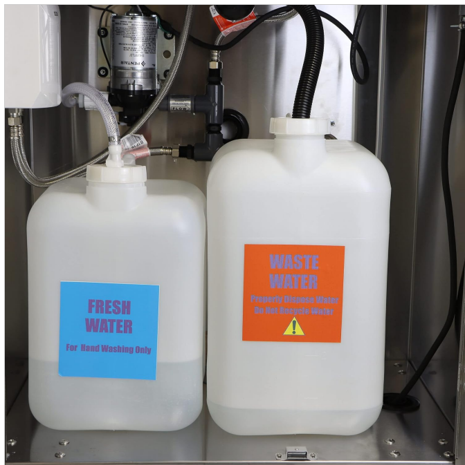
Figure 2: Fresh and waste water tanks inside the cabinet.
