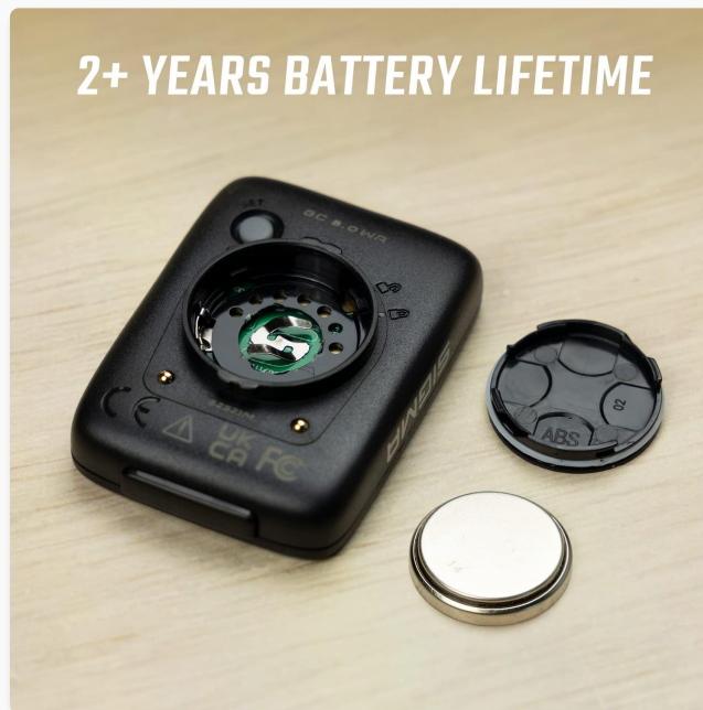
Image 5.1: The battery compartment of the BC 8.0, showing the replaceable CR2032 battery.
