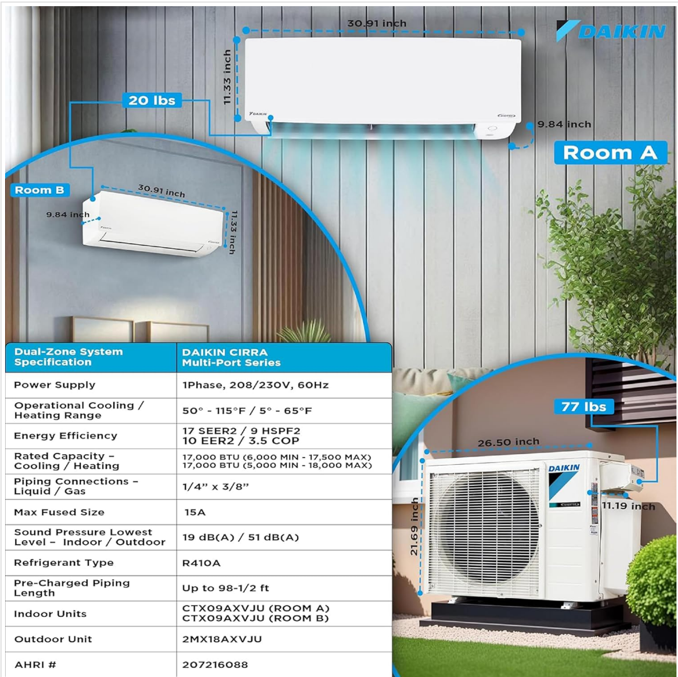
Figure 6.1: Detailed diagram showing dimensions of both indoor and outdoor units, along with key specifications such as power supply, operating ranges, rated capacity, piping connections, refrigerant type, and pre-charged piping length.
