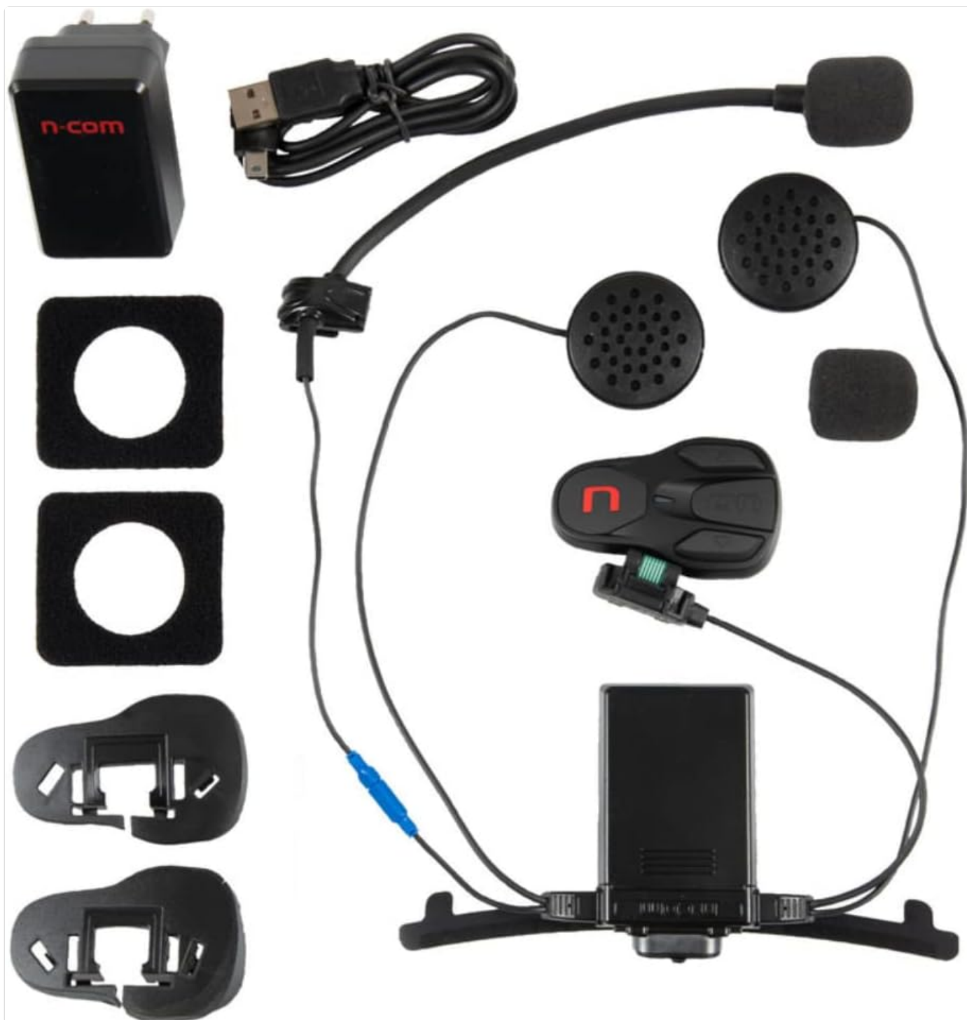
Figure 2: Included components of the Nolan N-Com B902 R system, including the main unit, speakers, microphone, and mounting accessories.
