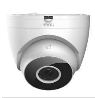
Figure 4.1: Front view of the IPC-T22AP camera, showing the lens and infrared sensors.
