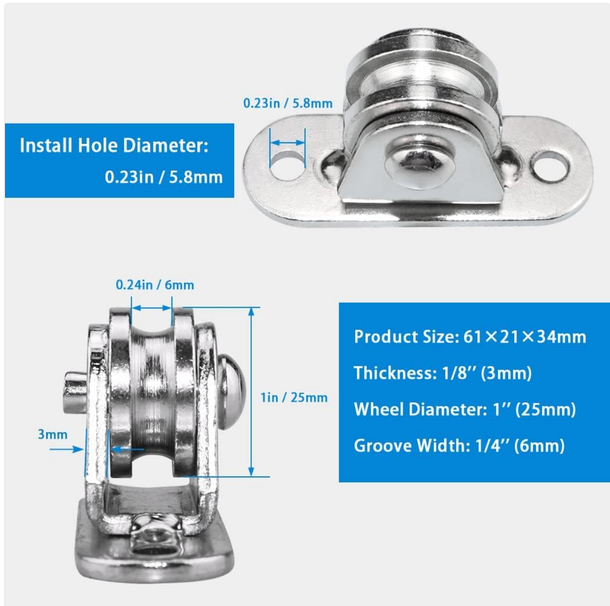
Image: This image provides a detailed breakdown of the pulley block's technical specifications, including its overall size (61x21x34mm), thickness (3mm), wheel diameter (25mm or 1 inch), and groove width (6mm or 1/4 inch). It also highlights the 5.8mm installation hole diameter.
