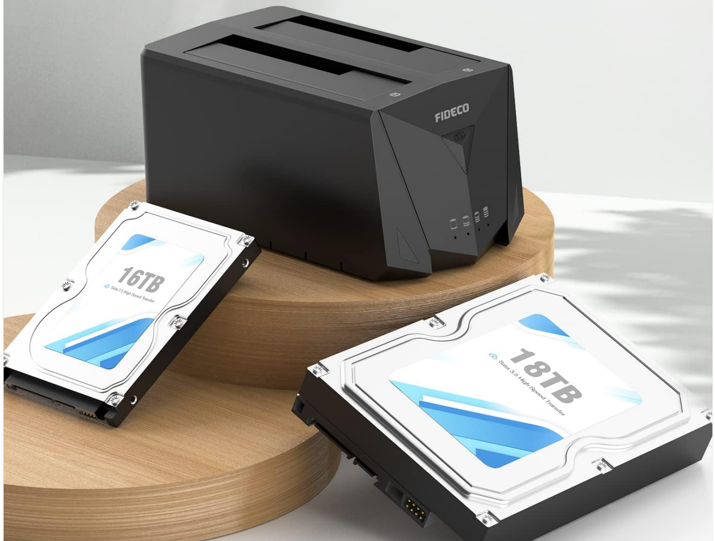
Image 4.1: Illustrates inserting 2.5-inch and 3.5-inch SATA drives into the docking station.
