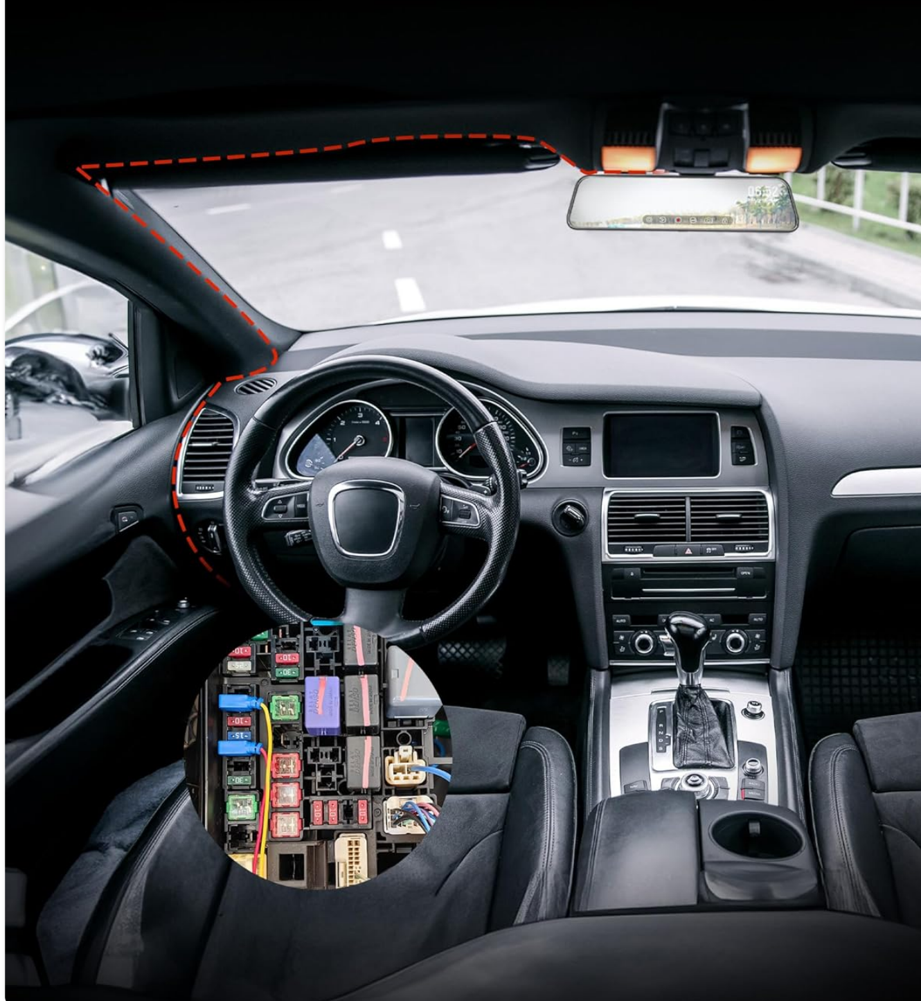
Image: Example of fuse box location and suggested cable routing in a car interior.
