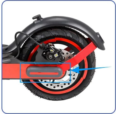
Step 02: Remove the side reflectors
