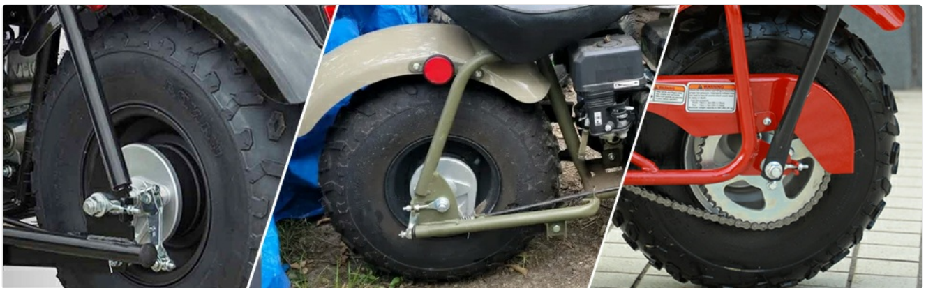
Image 5.2: Various mini bike rear axle configurations where the tensioner can be installed.
