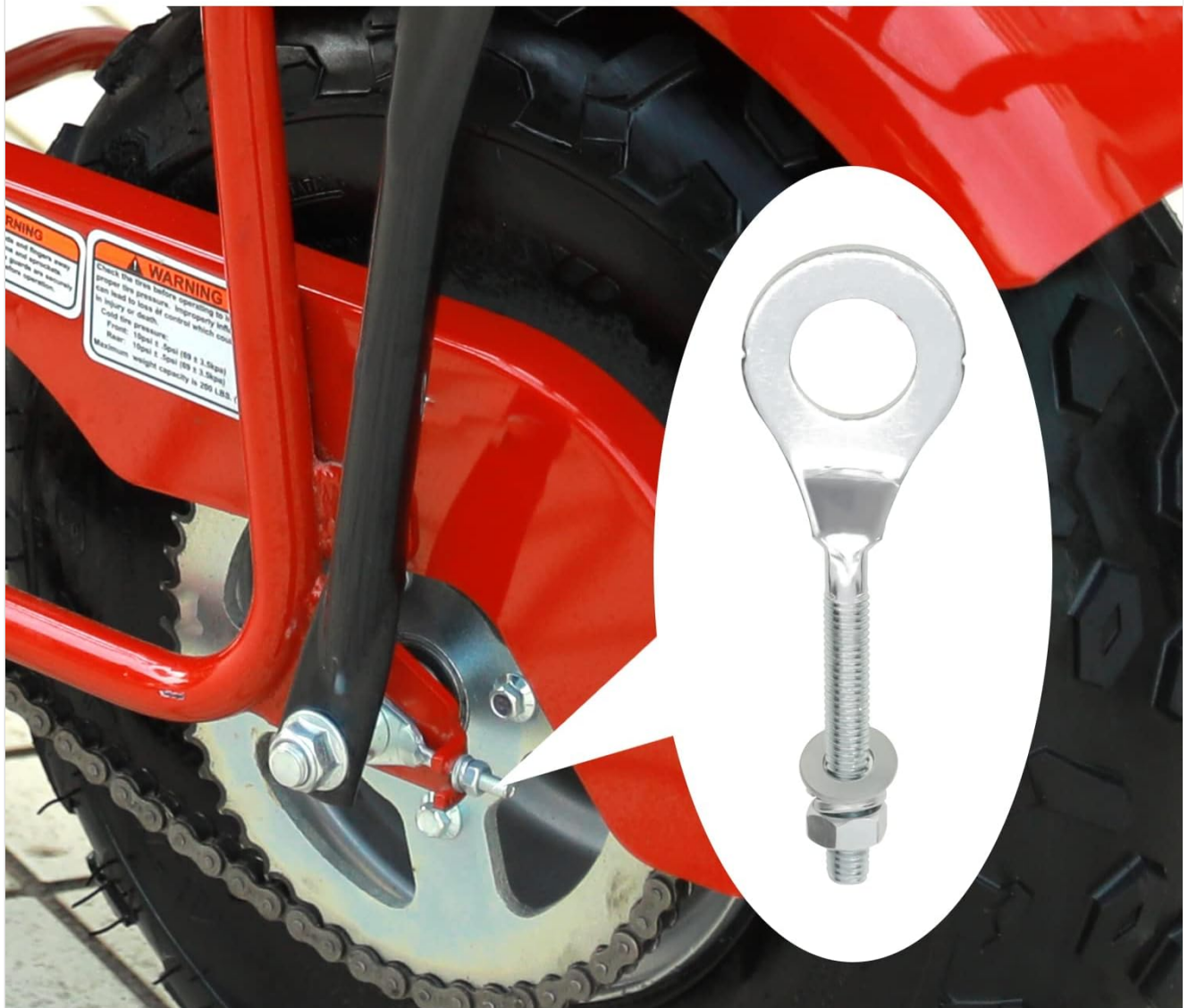
Image 5.1: Example of a chain tensioner installed on a mini bike.
