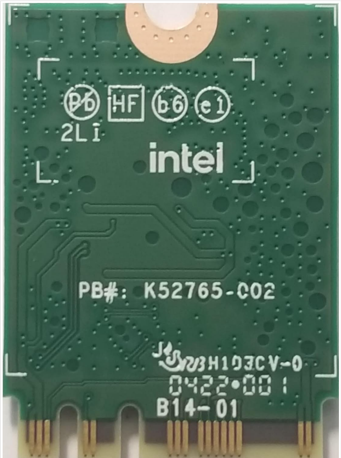
Figure 1: Front view of the Intel AX210 Wi-Fi/Bluetooth Combo Adapter, highlighting the model number and connection points.
