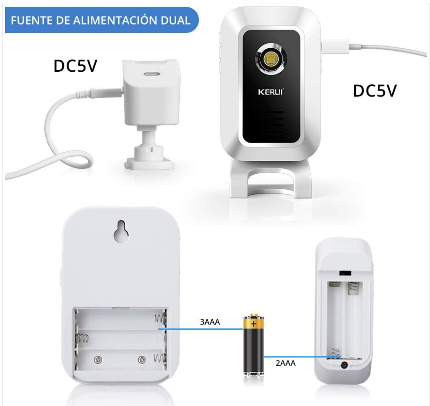
Figure 3: The KERUI M7 receiver can be powered via a DC 5V adapter or 3 AAA batteries. The PIR sensor typically uses 2 AAA batteries.
