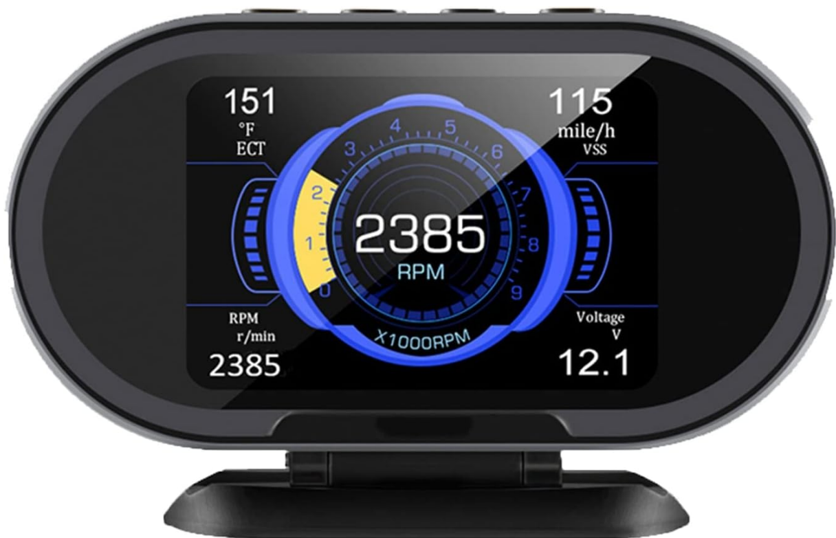
Image: The TSUSF KW206 display unit, showing various real-time vehicle parameters such as RPM, speed, engine coolant temperature, and battery voltage.
