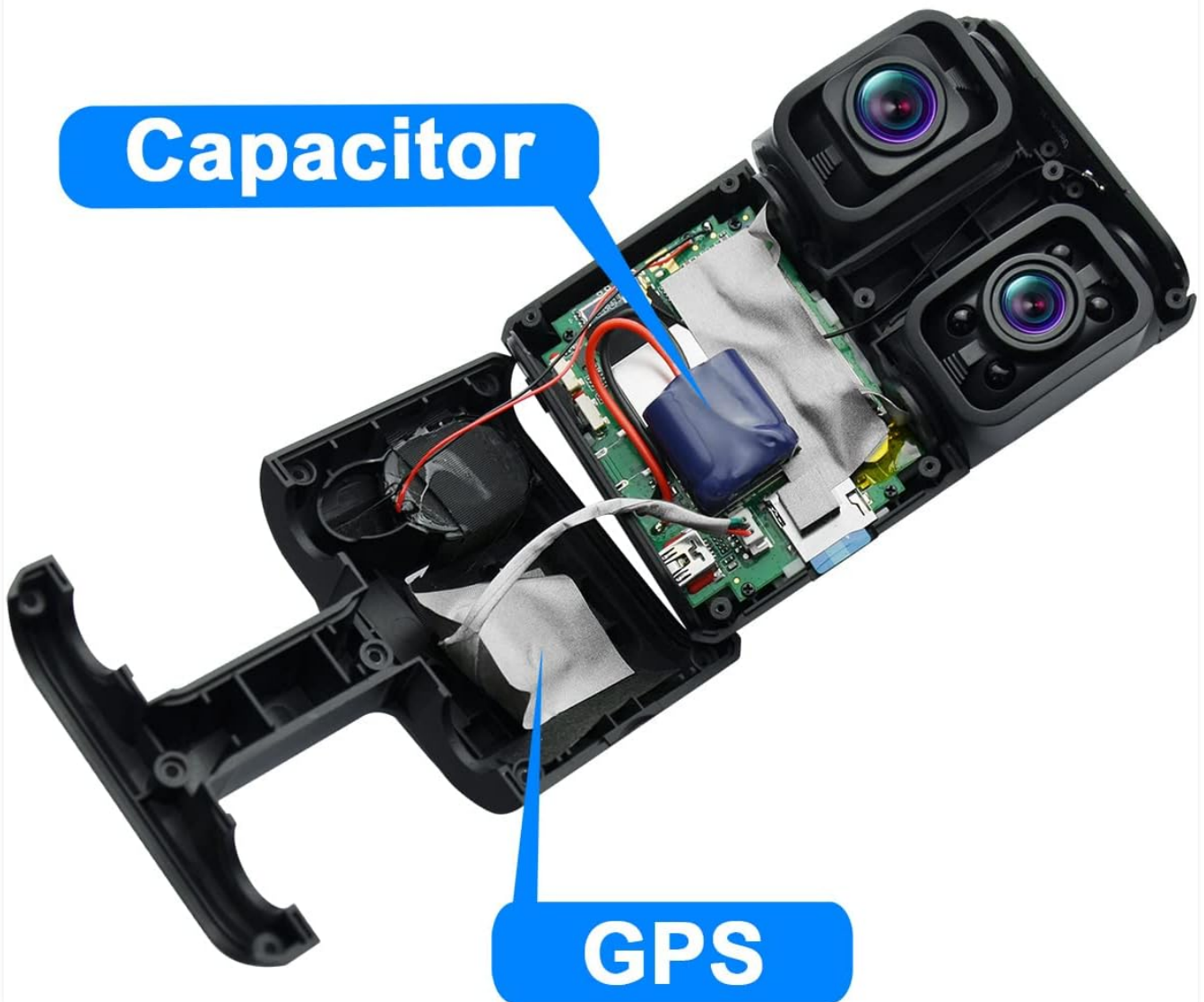
Image 4.4: An internal view of the dash cam, highlighting the integrated GPS module and capacitor for reliable operation.
