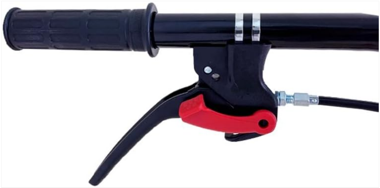
Image 4.2: Close-up of the clutch lever with its safety mechanism on the SAKAWA 1G72 Tiller handlebar.
