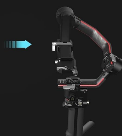
Figure 3.3: Quick disassembly and mode switching of the quick release plate.
