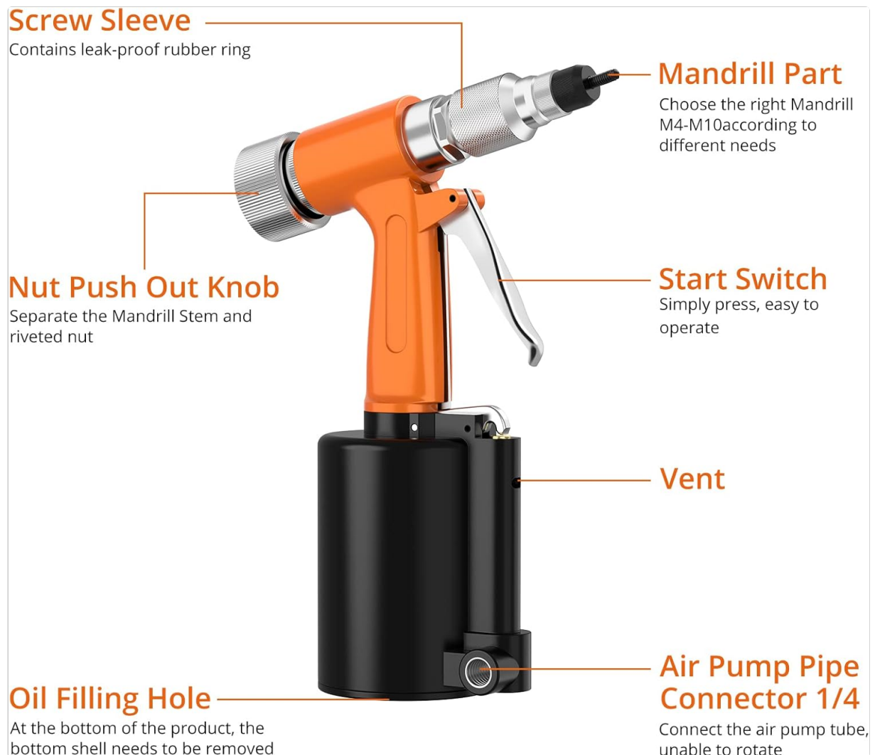
Image: Labeled diagram of the pneumatic rivet nut gun, highlighting key parts for identification and function.
