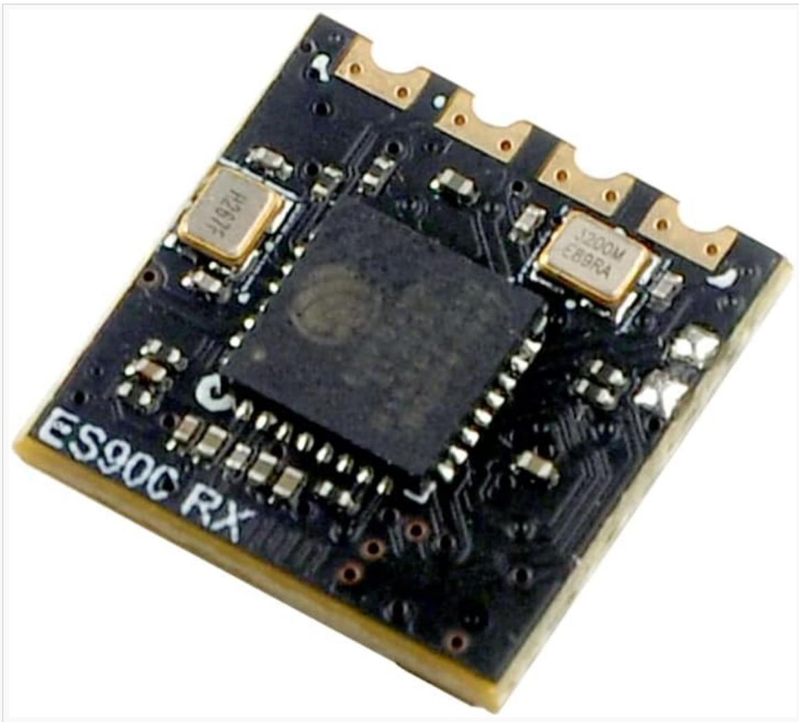
Figure 3.3: A detailed close-up view of the ES900RX module, highlighting its compact design and component layout. The module is designed for minimal footprint in FPV builds.
