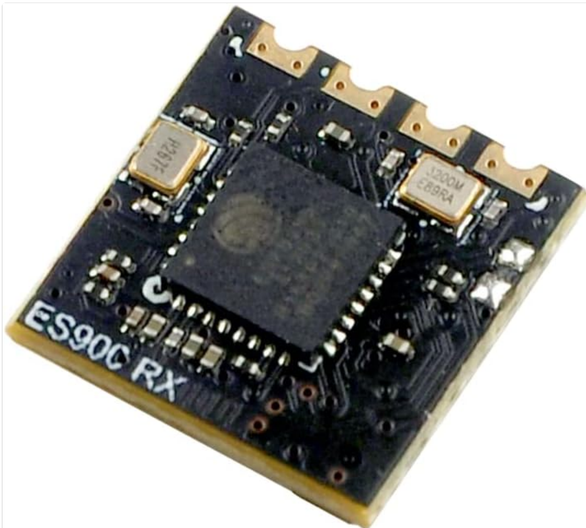
Image 3: A detailed close-up view of the compact HAPPYMODEL ES900RX Receiver Module.
