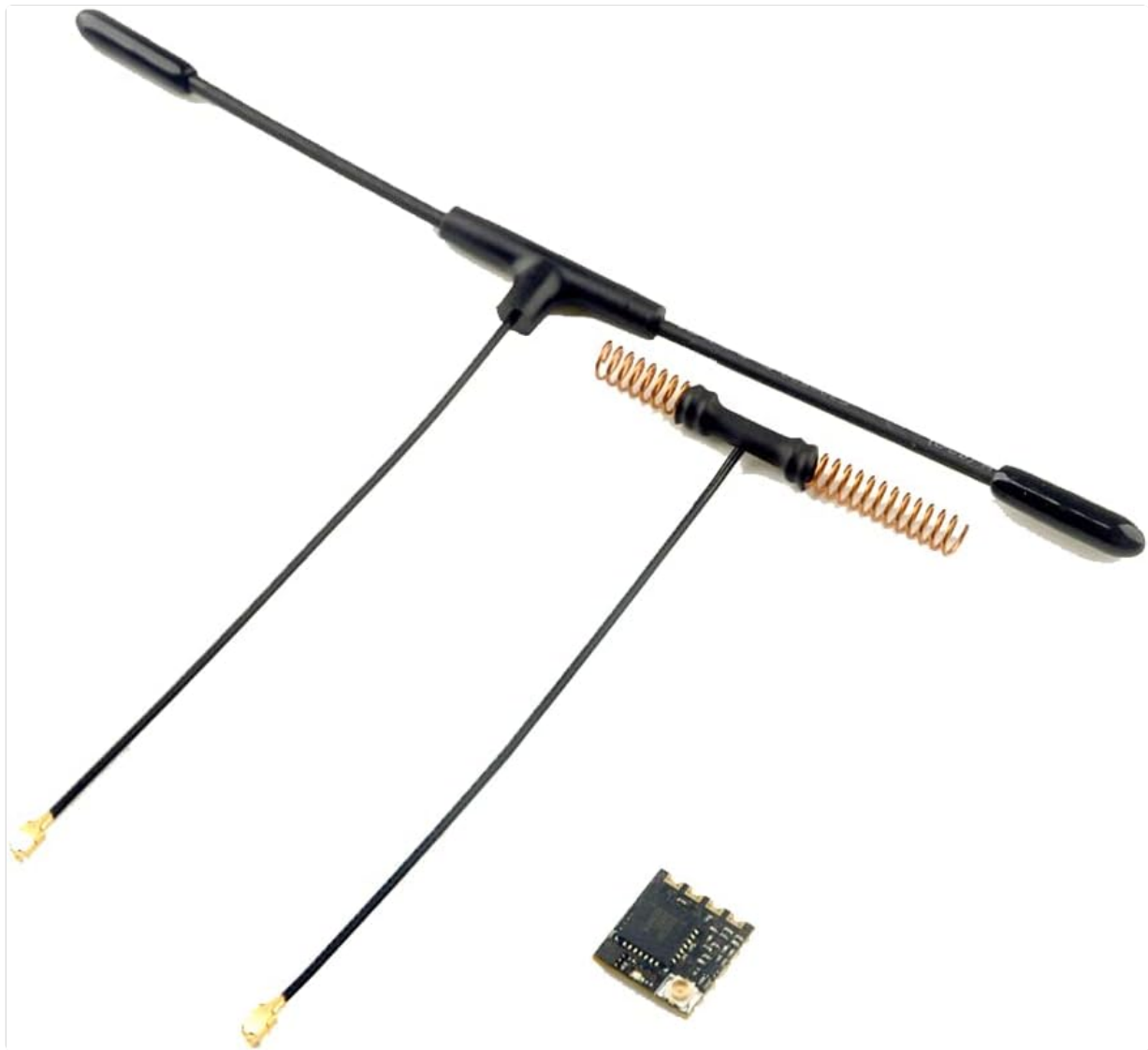
Image 1: The HAPPYMODEL ExpressLRS ES900RX 868MHz Receiver Module shown with its associated antennas.
