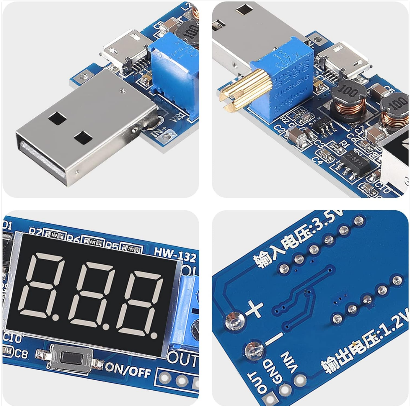
Figure 3: Detail of the Potentiometer and Display.
