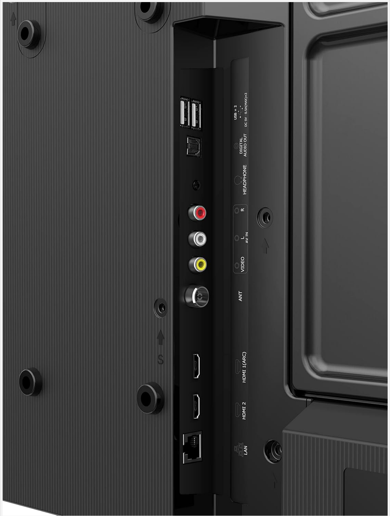
Image: Detailed view of the Hisense TV's rear panel, showing various input and output ports including HDMI, USB, LAN, and audio connections.
