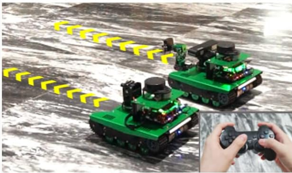
Figure 2.1: Overview of Transbot model options, including 3 DOF robotic arm, Astra Pro Plus depth camera, SLAM A1 Lidar, and 7-inch HD touch screen.
