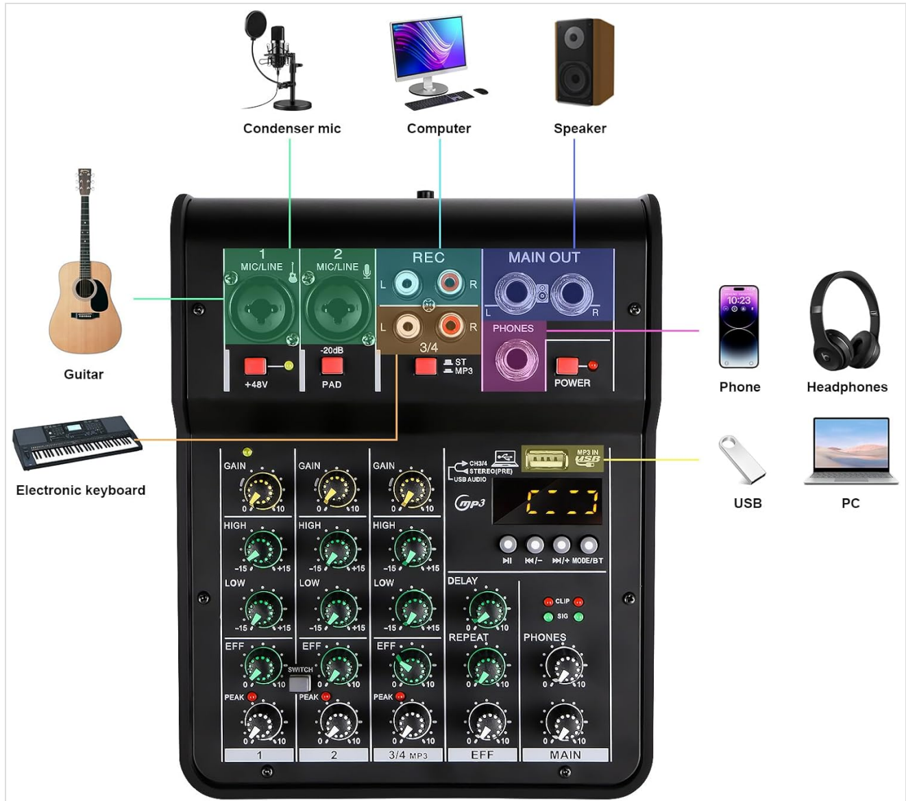
Figure 4.1: Diagram illustrating various device connections to the M4 mixer, including microphones, instruments, computers, and speakers.
