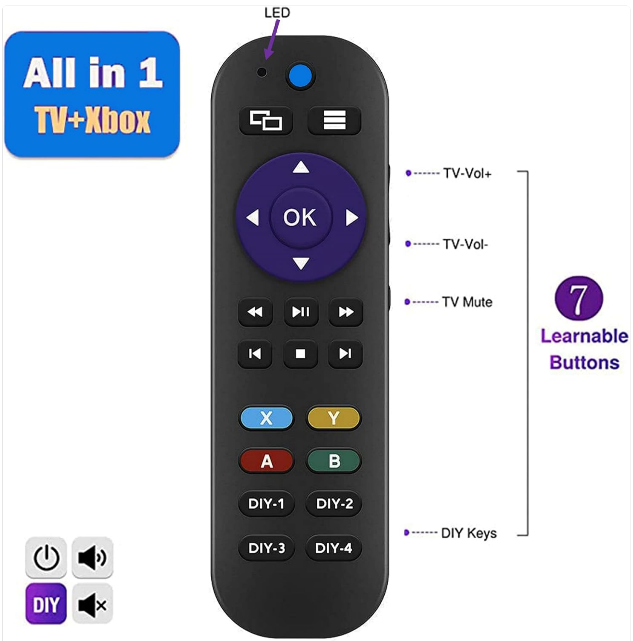
Image: A close-up of the Smartby Universal Remote highlighting the "TV-Vol+", "TV-Vol-", "TV Mute", and "DIY Keys" (DIY-1, DIY-2, DIY-3, DIY-4) as the 7 learnable buttons.
