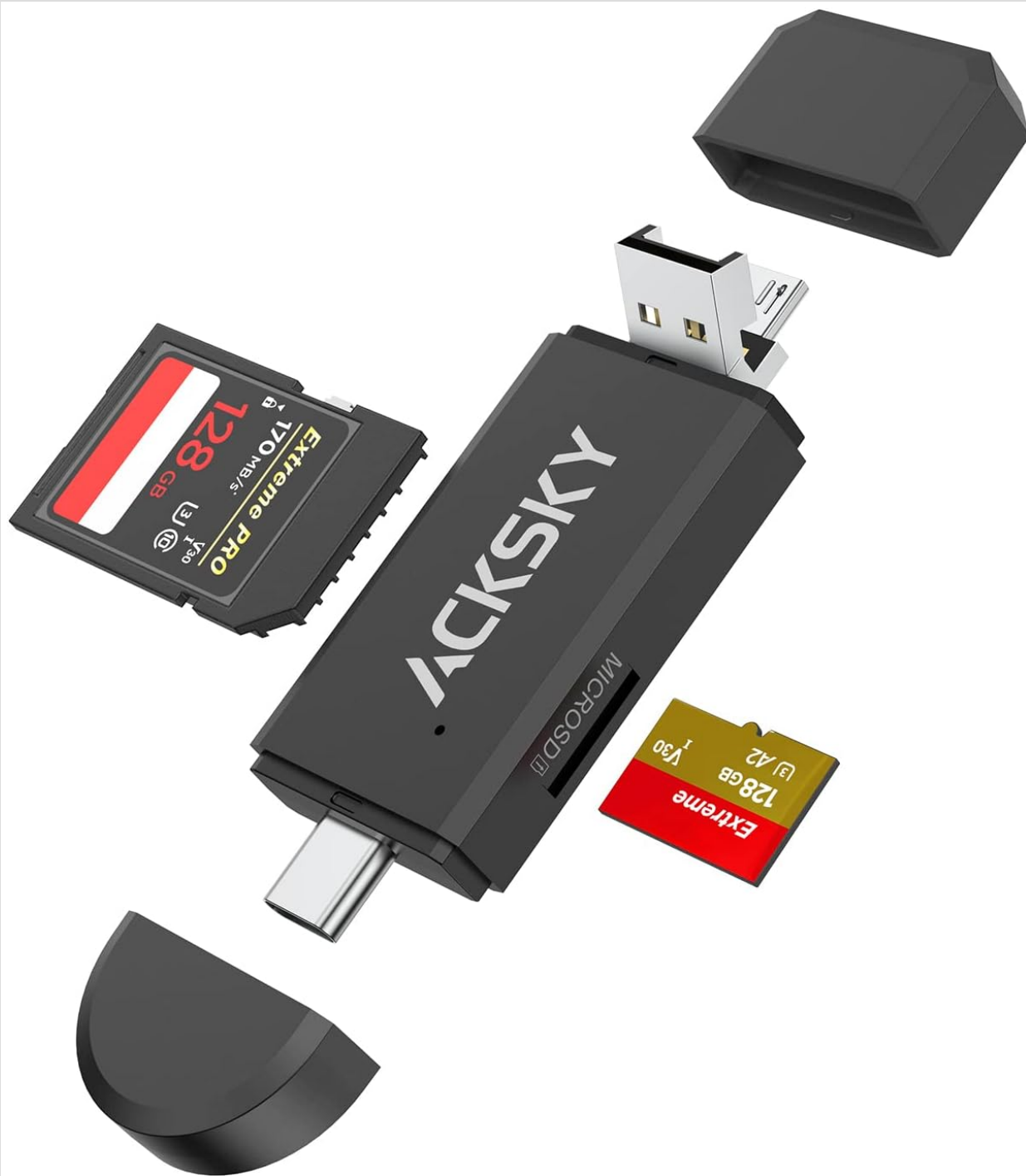
Image 1.1: The ACKSKY 3-in-1 SD Card Reader, showcasing its USB-A and USB-C connectors, along with slots for standard SD and Micro SD cards.
