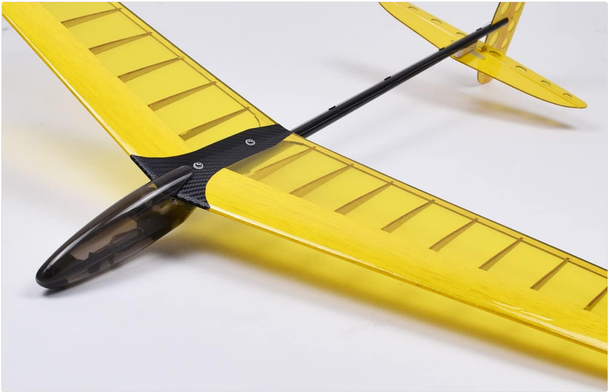
Figure 2: Fuselage with quick-release canopy for component access.
