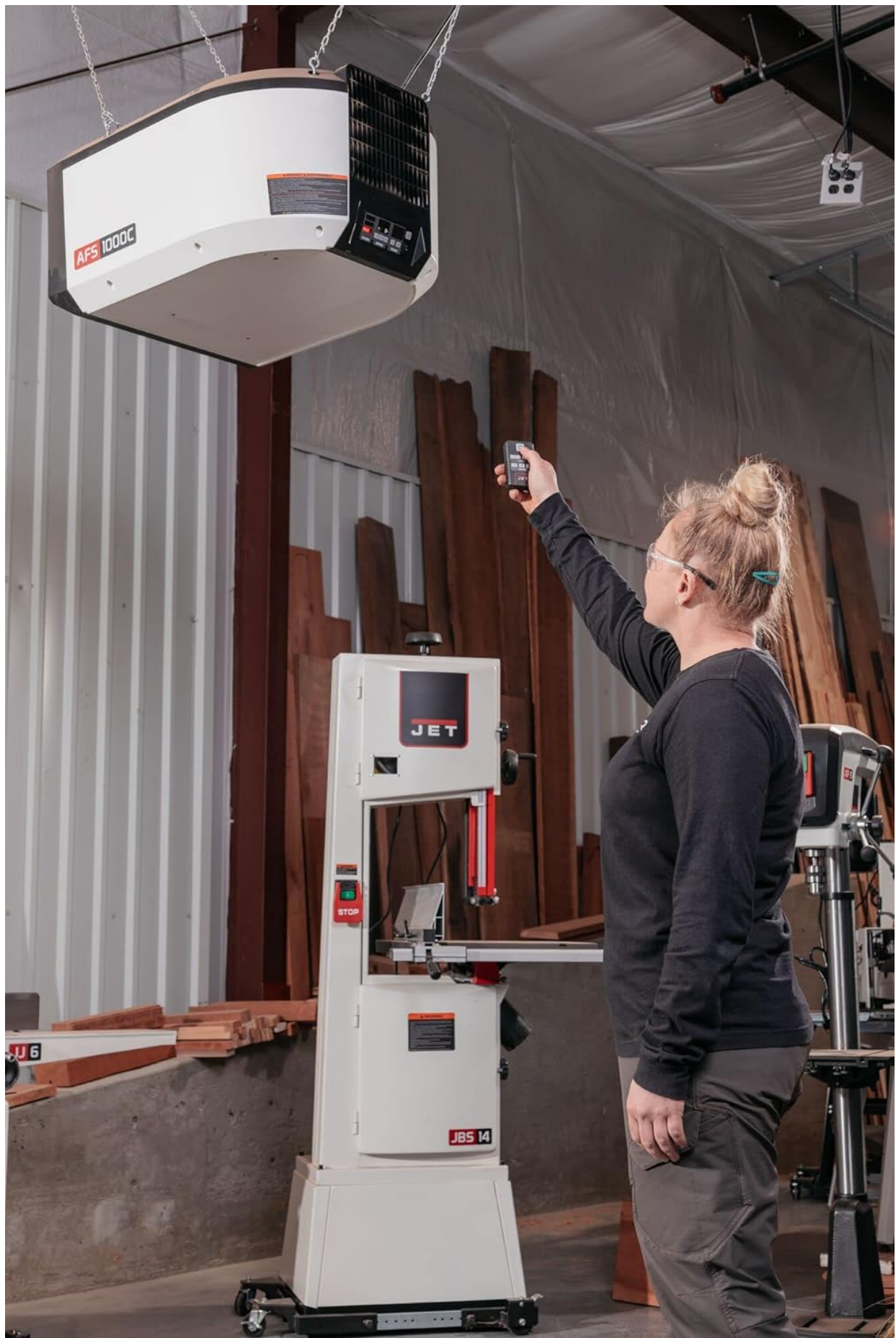
Figure 4.1: The AFS-1000C unit properly mounted in a workshop environment.
