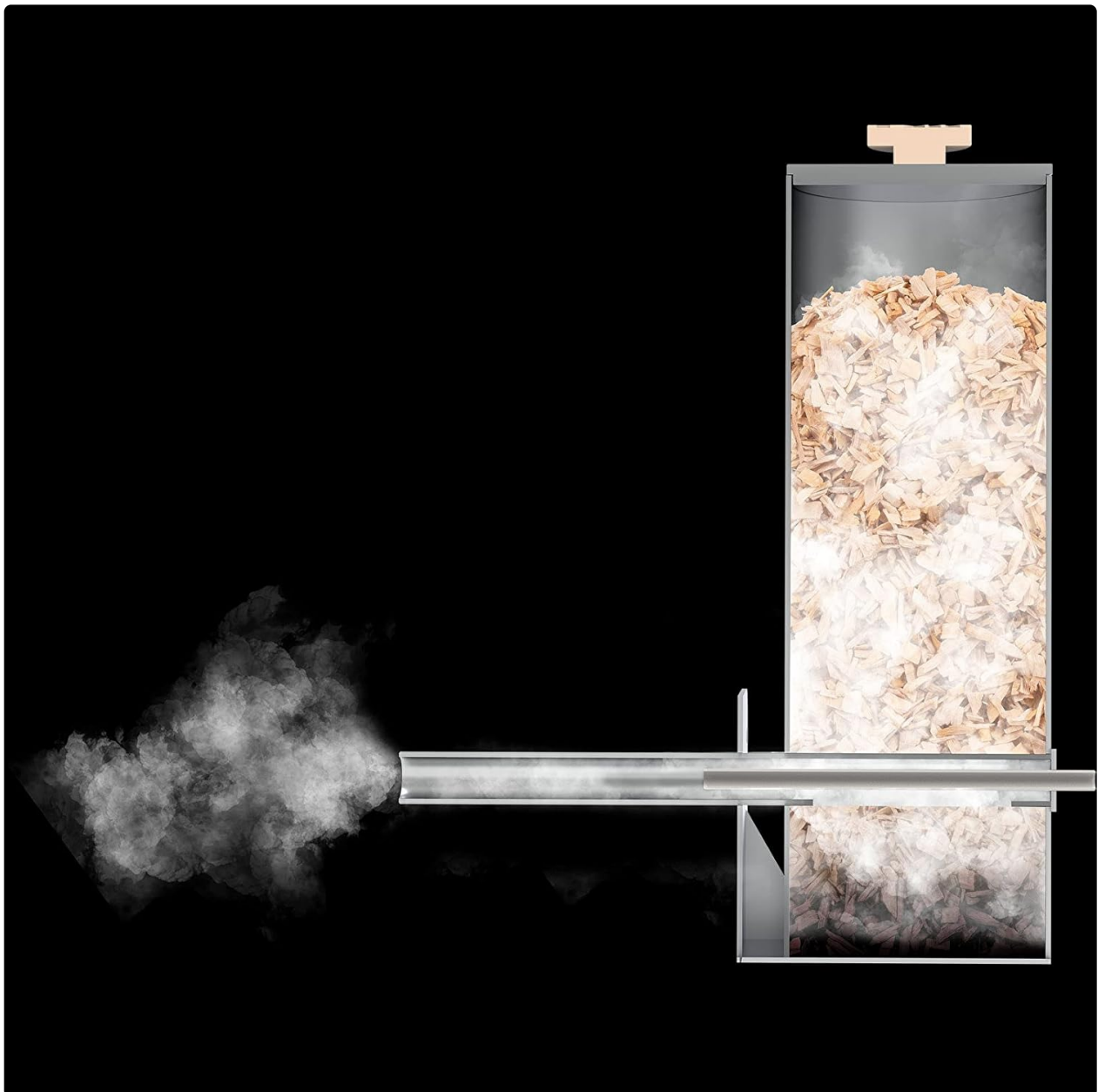
Image 5.1: Cross-section illustrating the wood chips inside the generator and the path of smoke being pushed out by the air pump.
