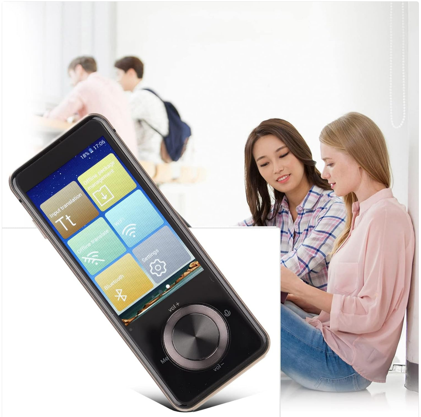
Figure 4.1: The translator's screen displaying various application icons, including options for input translation, offline package management, Wi-Fi, settings, Bluetooth, and offline translate.
