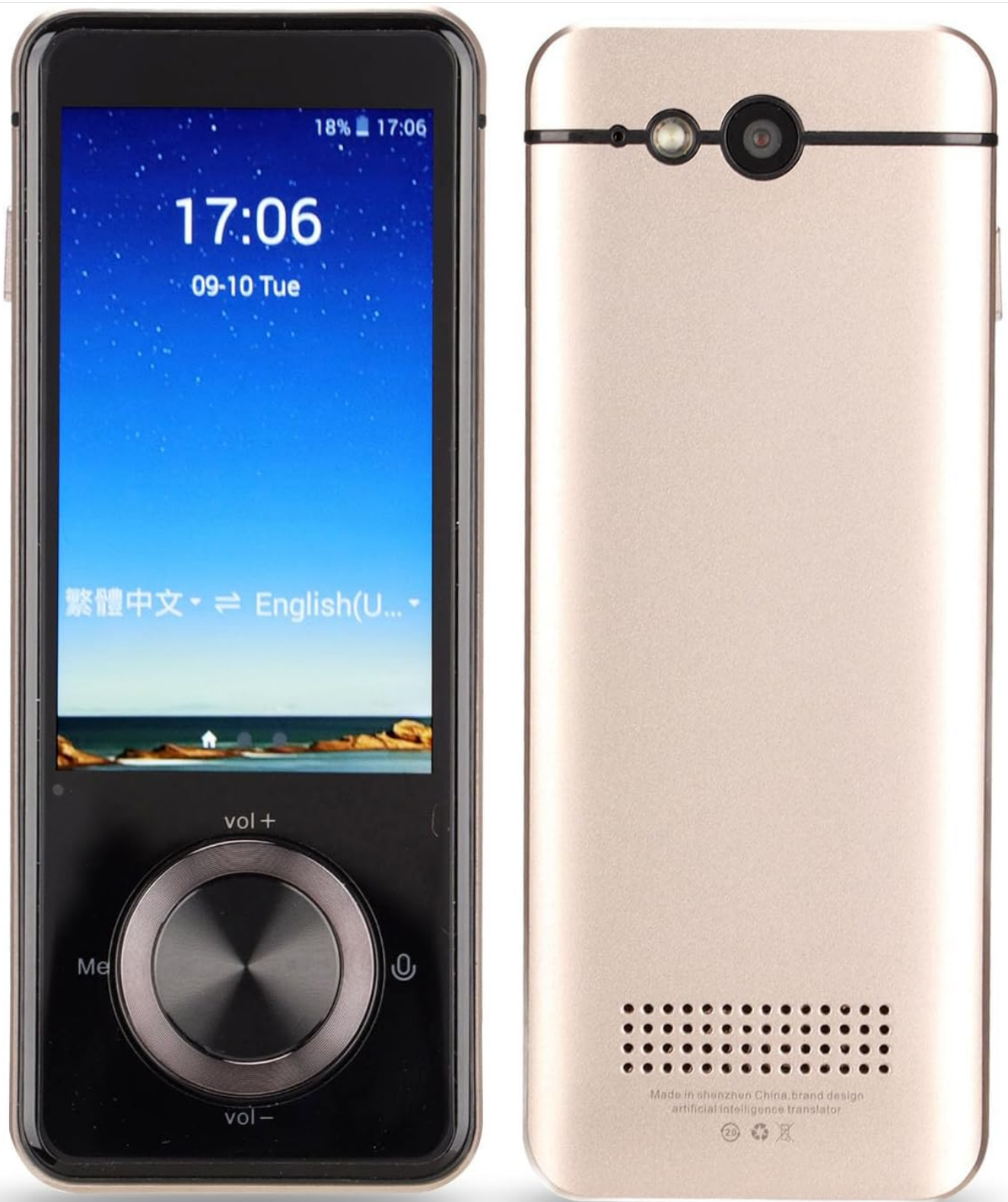
Figure 1.1: Front and back view of the ASHATA M9 Smart Instant Language Translator. The front features a 3-inch touchscreen and a circular control dial. The back shows the camera lens and speaker grille.
