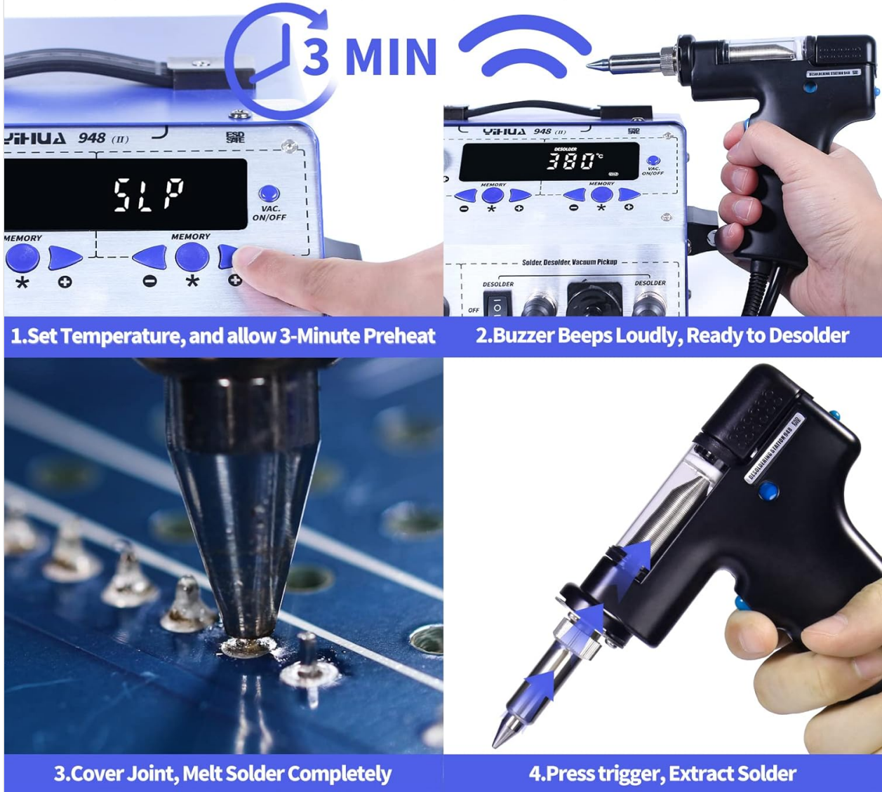
Figure 5: Step-by-step guide on how to use the desoldering gun, from setting temperature to extracting solder.
