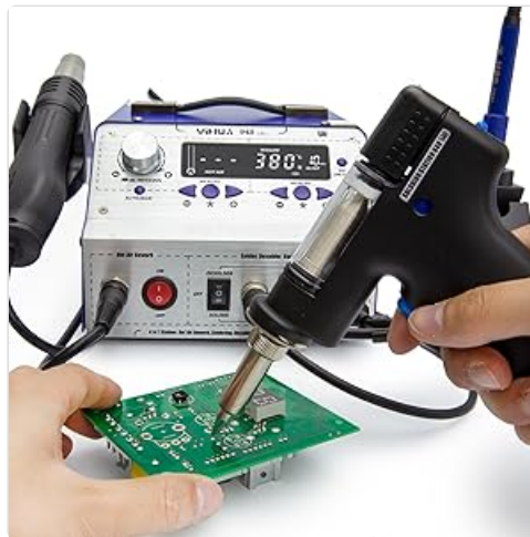
Figure 4: Illustration of the hot air gun's automatic mode (cooling down in holder) and manual mode (continuous operation).
