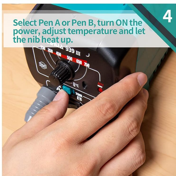
Image: Steps 1-4 of the pyrography process, from wood preparation to temperature adjustment.
