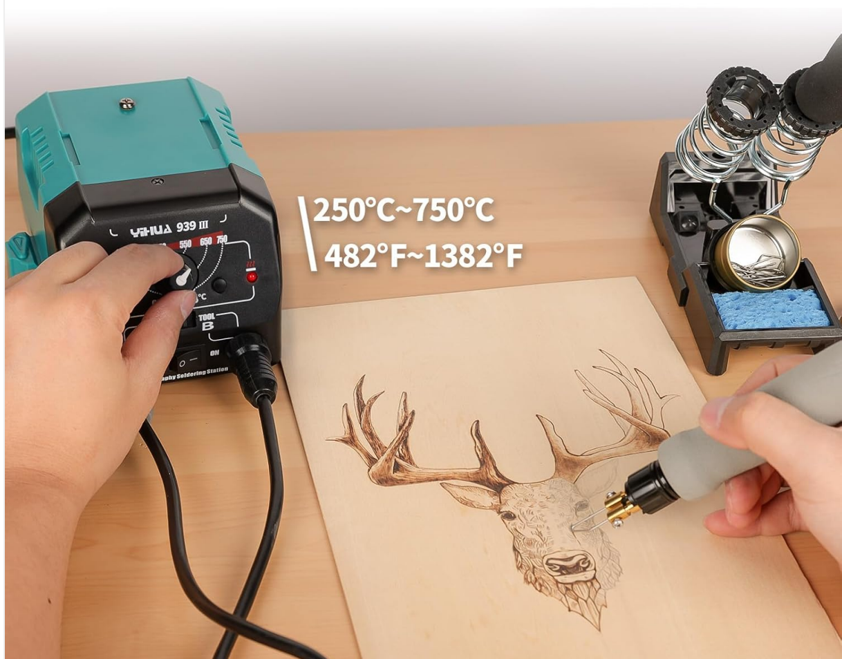
Image: Adjusting the temperature on the pyrography station.
