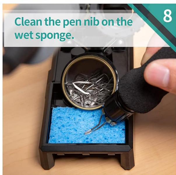
Image: Steps 5-8 of the pyrography process, including practice, tracing, power off, and cleaning.
