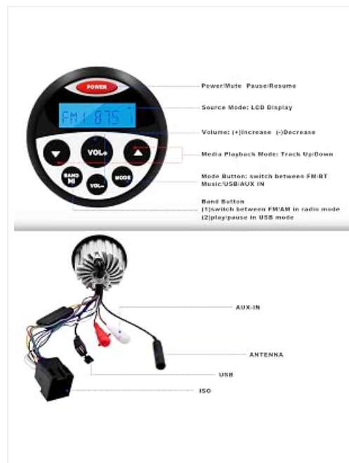
Figure 5.1: Front panel controls and their functions.
