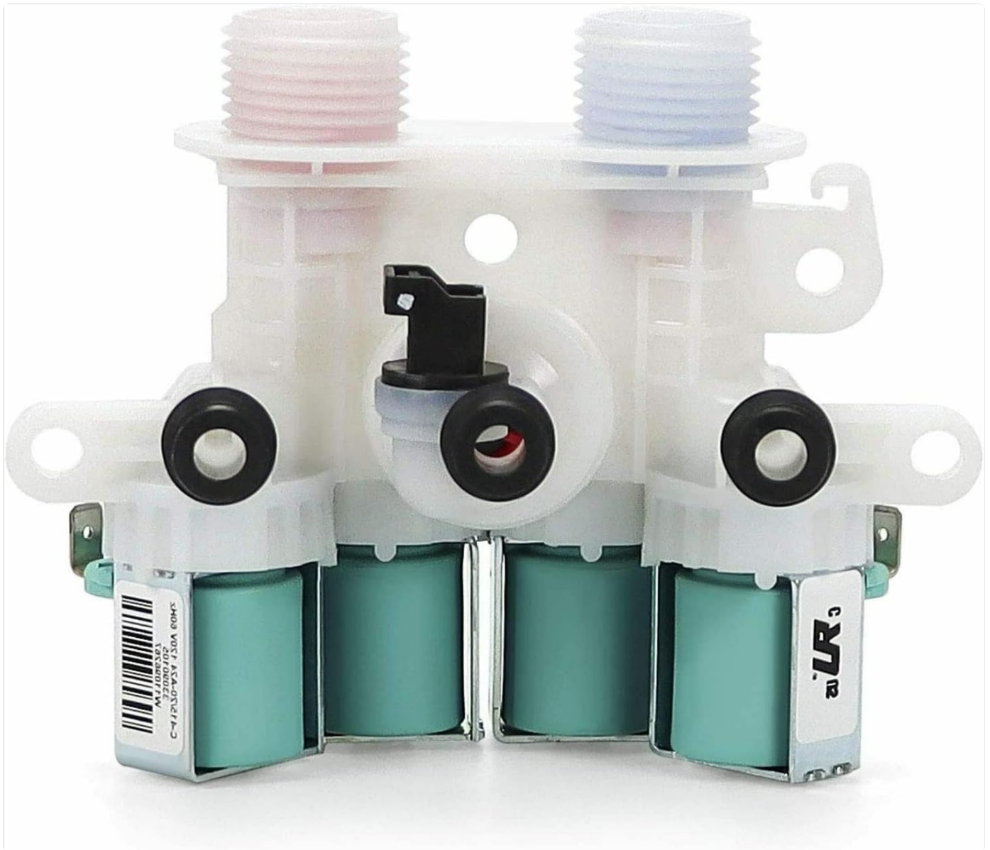
Figure 1: Owigit Washer Water Inlet Valve. This image displays the complete water inlet valve assembly. It features two threaded inlet ports, one for hot water (indicated by a red-tinted thread) and one for cold water (indicated by a blue-tinted thread), located at the top. Below these are the solenoid valves, which are typically green or teal in color, responsible for controlling water flow. The valve body is made of white plastic, with black rubber seals around the outlet ports. The overall design is compact, intended for direct replacement in compatible washing machines.
