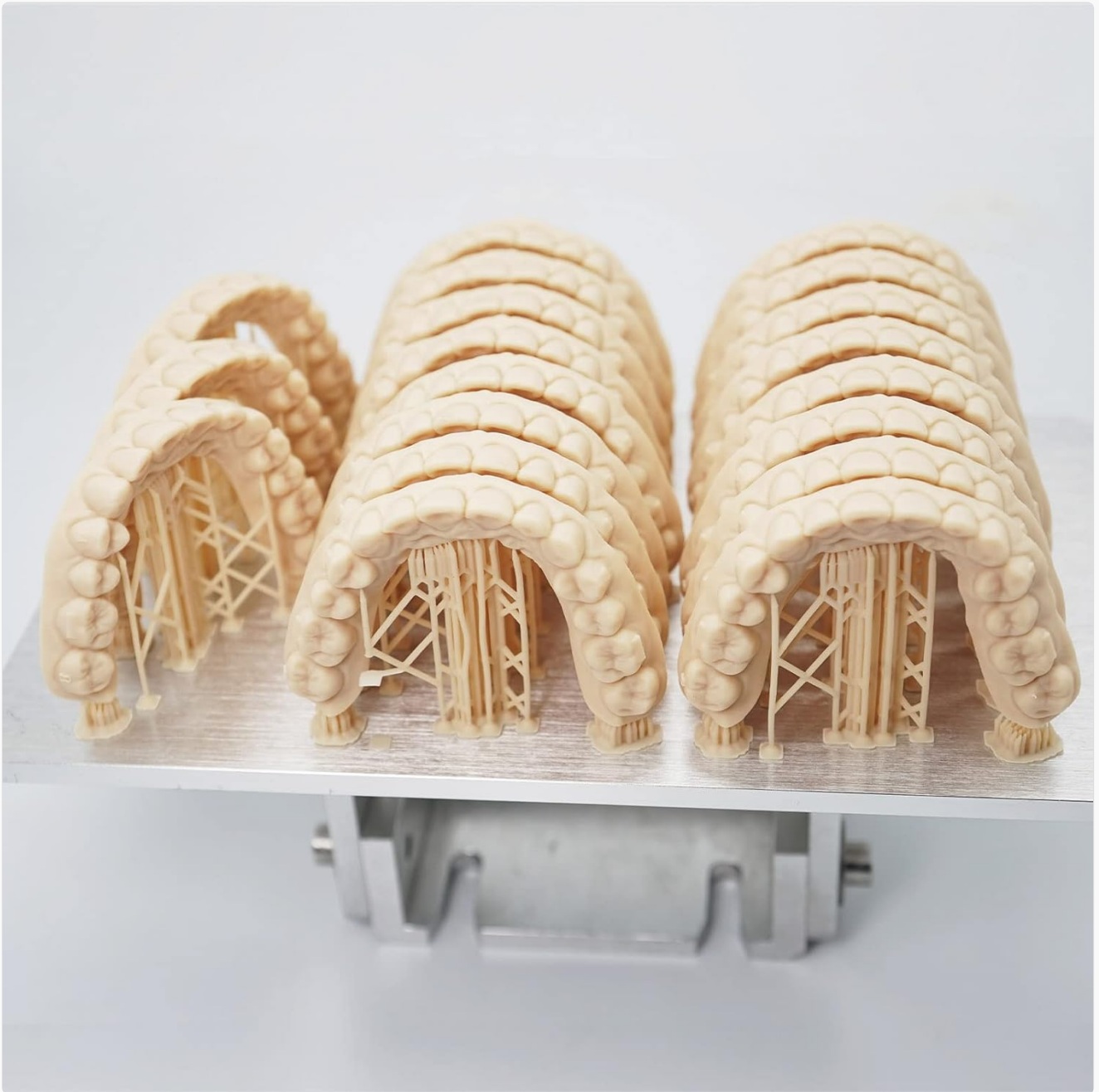
Image: A batch of 3D printed dental arches still attached to a build plate, demonstrating the resin's capability for producing multiple detailed models simultaneously.
