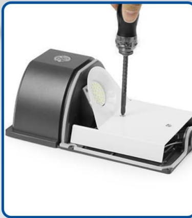
2. Loosen 2 screws enough to allow reflector to slide upward until keyhole reflector releases from 2 screws. Remove reflector.
