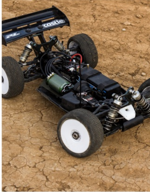
Image: A close-up view of the Mamba Micro X2 ESC installed within an RC buggy chassis, showing wiring connections.
