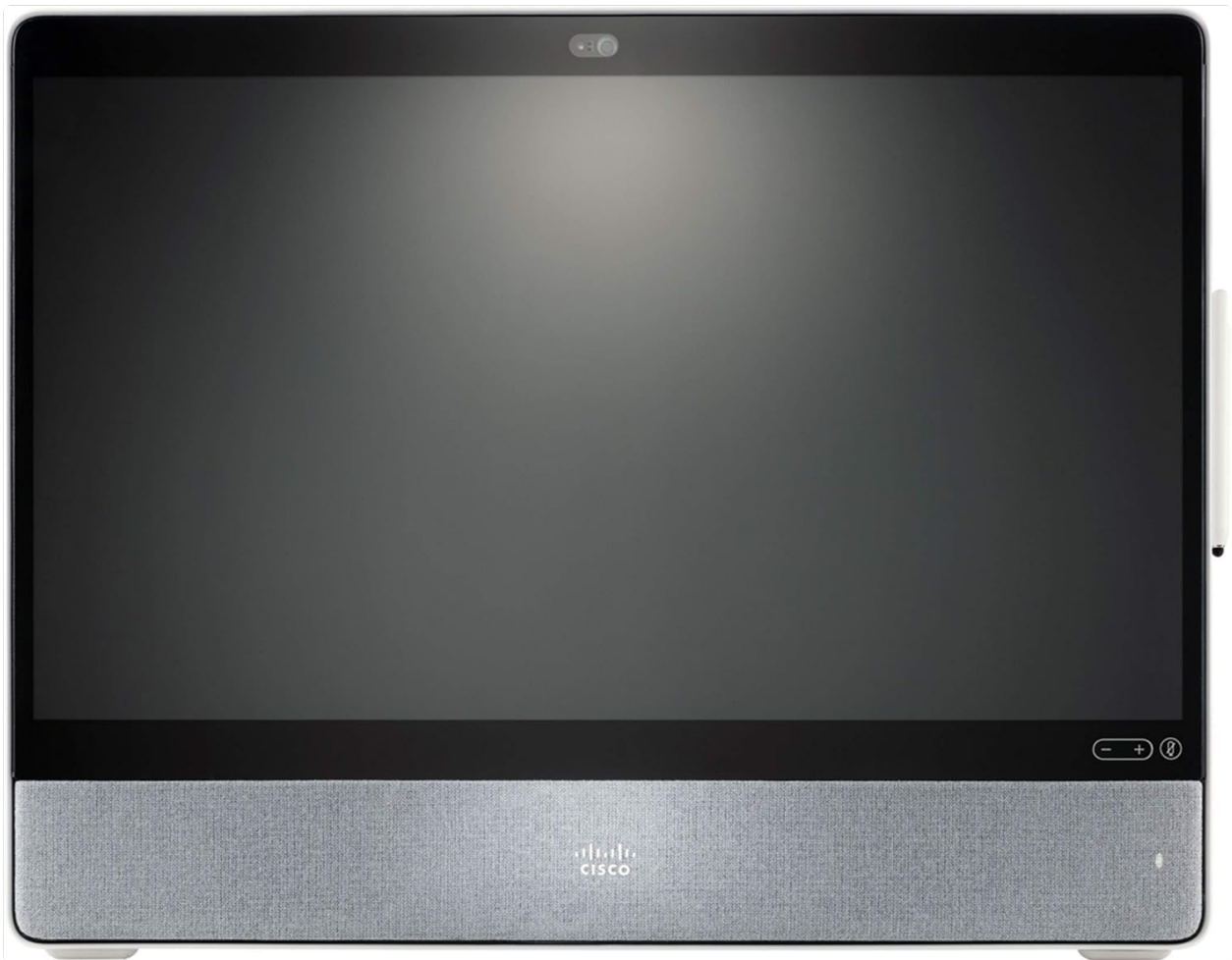
Figure 2.1: Front view of the Cisco Webex Desk Pro, showing the 27-inch display, camera, and speaker grille.
