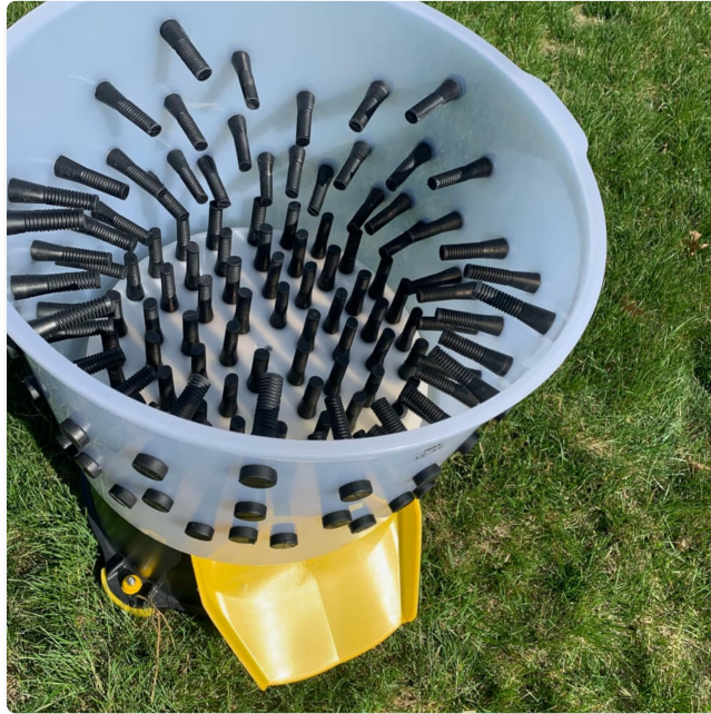
Figure 5: Interior of the plucker drum with plucking fingers.
