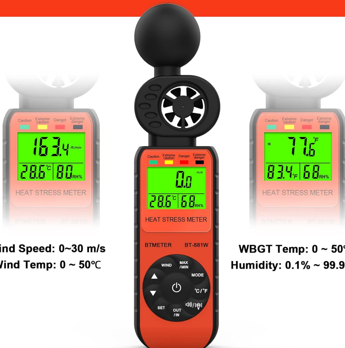
Figure 5: The BT-881W provides visual indications for different WBGT hazard levels: Caution (26.7-29.4°C), Extreme Caution (29.4-31°C), Danger (31-32.2°C), and Extreme Danger (>32.2°C).
