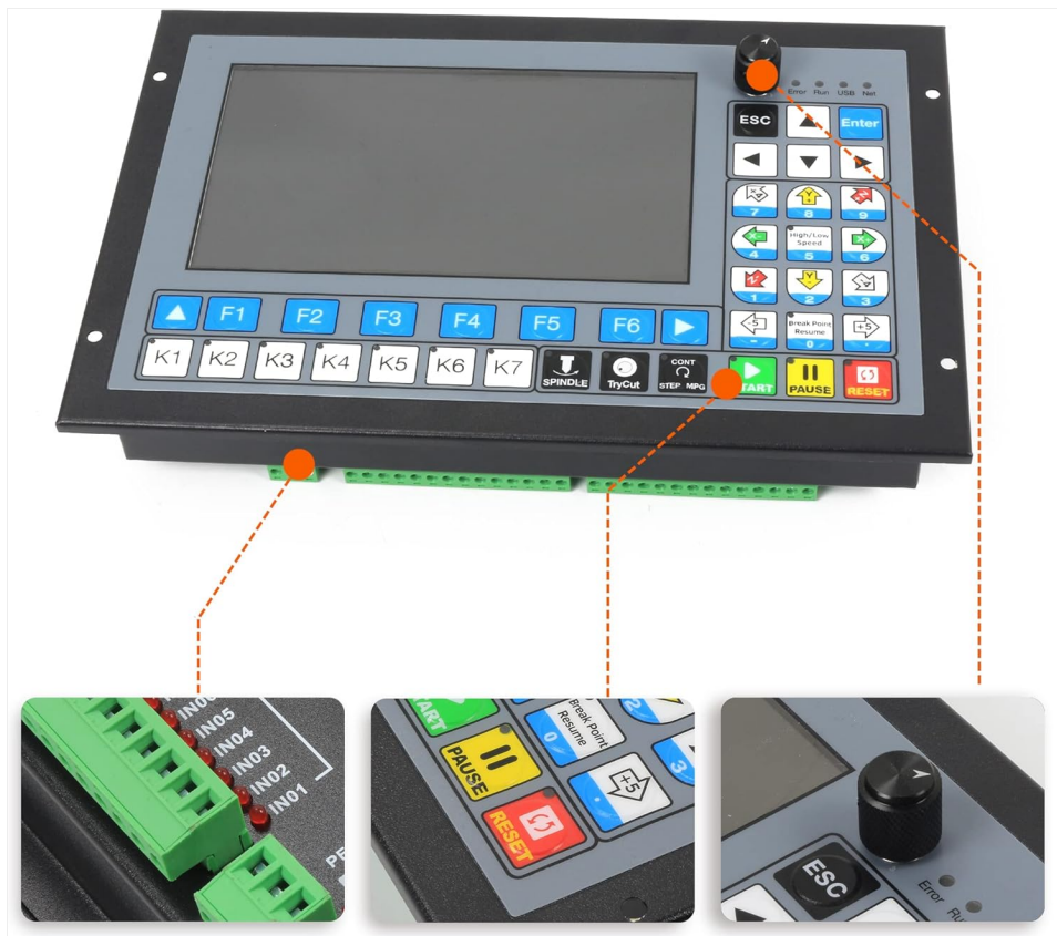
Figure 5.1: Close-up view of the controller's front panel, highlighting key interface elements.
